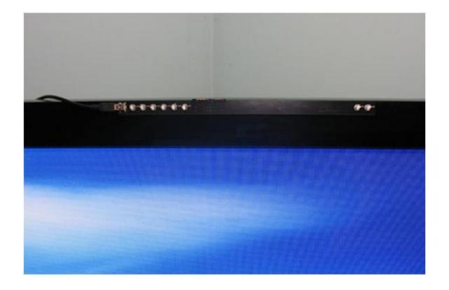
The Super Light Bar needs to be mounted near the top of the TV/Monitor as shown in the picture above. Notice how the USB cable is coming out of the LEFT side of the light bar (This is important). The light guns will not operate correctly if the light bar is mounted upside down or near the bottom of the TV/monitor.
